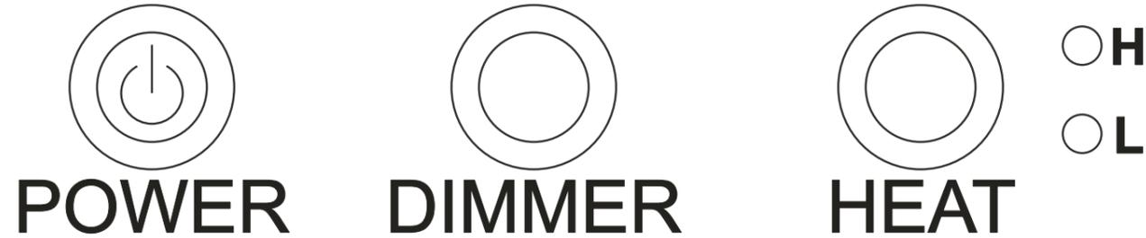
To begin operation touch the Power button. The flame image and fire feature will be on at full brightness and the heater will be off.
