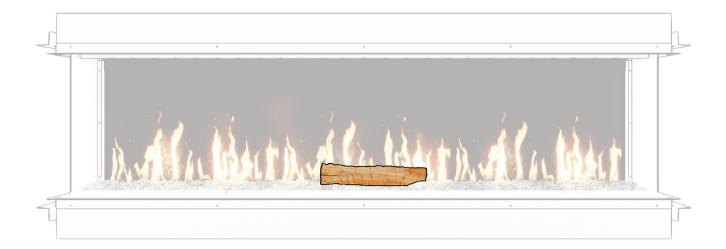
Select the two 16" side logs and rest them on the left and right of the base log. These are now creating the main portion of your stack. Spreading these out more for linear shaped fireplaces and bringing these closer together for traditional shaped fireplaces.
