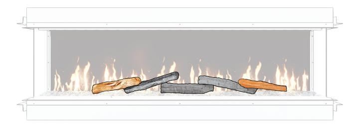
4. Select the 12" slim logs and lay them under the 12" large logs. The inside end of the log may be towards you and the outside end may be towards the flame screen.
