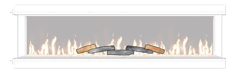
4. Select the 12" slim logs and stack these on the ends of the 12" big logs.
