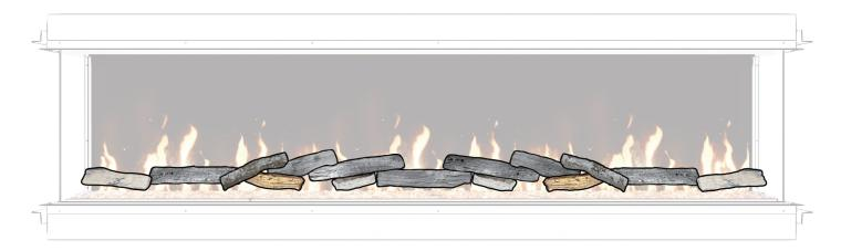
9. Select the 10" logs, and stack these laying over the 16" filler logs. The inside end of the log may be towards you and the outside end may be towards the flame screen.
