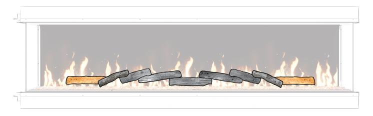
6. Select the last two of the 12" big logs, and lay these near the 16" filler logs. The inside end of the log may be towards you and the outside end may be towards the flame screen.
