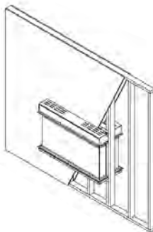
Floating 2x4 Wall Installation
