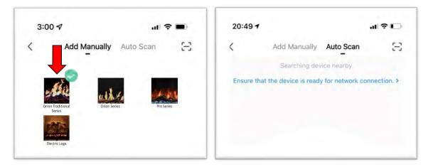
• On the fireplace touch controls, press and hold the "Flame" button for 5 seconds. The fireplace will show either "P0" or "P2". This will place the fireplace in pairing mode.
