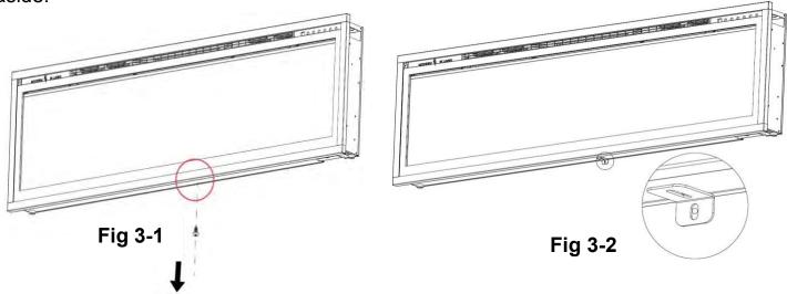
**B.**Using the screw previously removed, attached the L-bracket (**O**) (supplied) to the bottom of the fireplace box.(Fig 3-2)
